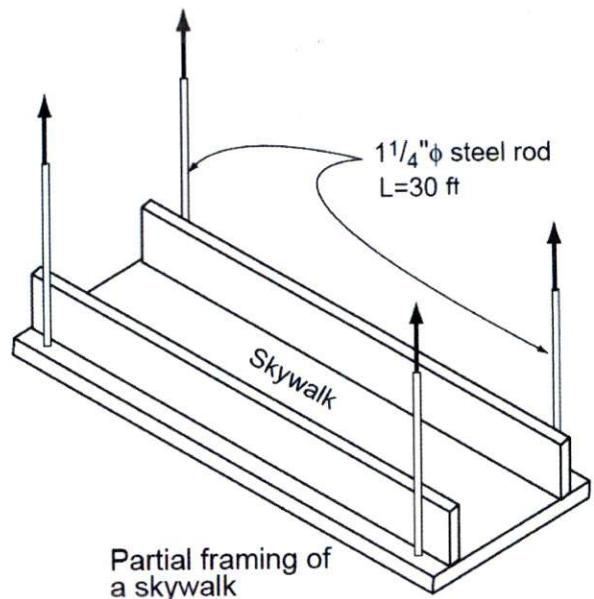
(b) if the rods supporting the skywalk are 30 ft in length , how much elongation would occur if the rod was loaded to its maximum allowable Stress limit
